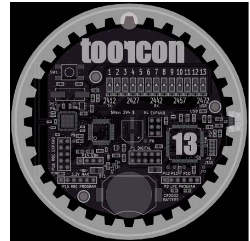
RF spectrum analyzer with LEDs representing 13 evenly spaced Wi-Fi channels in the 2.4 GHz band
